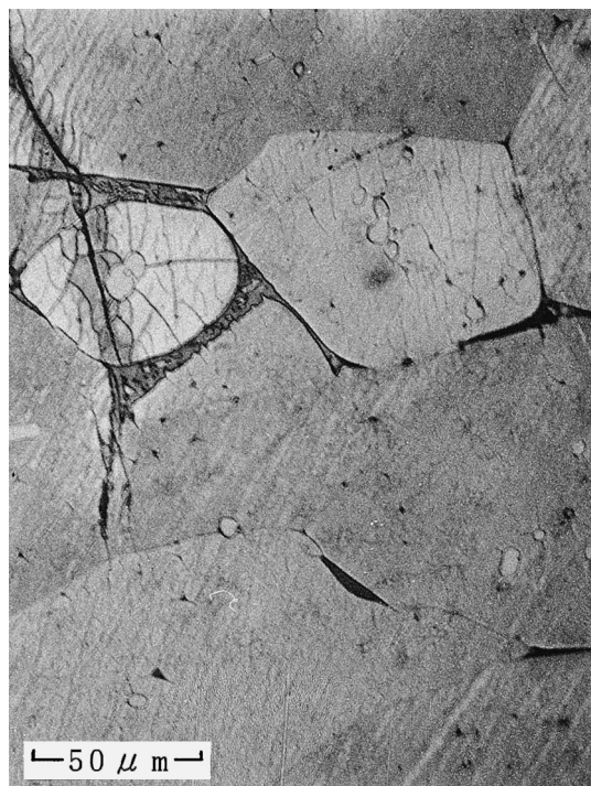
Fig. 5. Microstructure of U_3MoSi_2 ; the near-central part of Fig. 3 is enlarged. The 0.6 wt% Si-dissolved \gamma -(U, 8.4 wt% Mo) alloy precipitates along the grain boundaries of U_3MoSi_2 . An unidentified impurity phase is also present as small globules.
