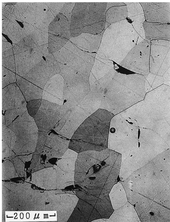
Fig. 7. Microstructure of pure \text{U}_3\text{Si}_2 alloy arc-melted and annealed at 850^\circ\text{C} for 4 days, showing single-phase \text{U}_3\text{Si}_2 (measured density = 12.2\text{ g/cm}^3 ).
